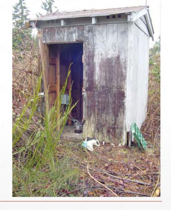
Well Depth - 60' Static - 48'6 Pump installed 17-8-98 3/4 49-12 gpra Gould Set on 1" poly Evergreen Jell Orilling
